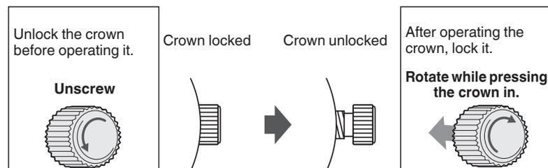
\* When locking the crown, turn it slowly with care, ensuring that the screw is properly engaged. Be careful not to push it in forcefully, as doing so may damage the screw hole in the case.
