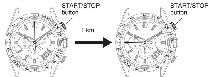
The measured result shows that the average speed of the vehicle is 80 km/h.
