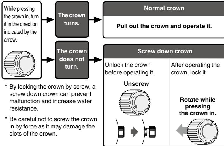
\* By locking the crown by screw, a screw down crown can prevent malfunction and increase water resistance.
