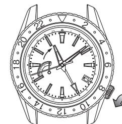
Turning the crown counterclockwise (6 o'clock direction): The hour hand is advanced one hour.
