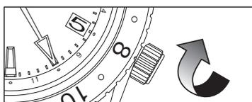
Turning the crown clockwise (12 o'clock direction):
