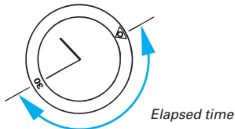
**1** Turn the rotating bezel to align the "▽" mark to the minute hand.
