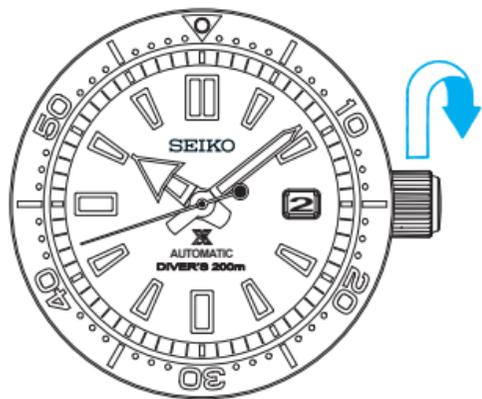
1. Slowly turn the crown clockwise (in the 12 o'clock direction) to wind the mainspring.
